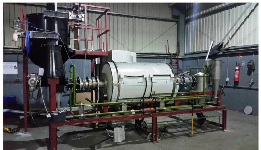
Within ReNEW a demonstration pyrolysis installation was developed to show the potential of this technology in harnessing inherent waste energy to generate value added products from different type of residuals. The capacity of pyrolysis unit is 50 kg/h of solid residues. The pyrolysis installation allows for process evaluation and scale up of the technology.
